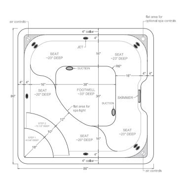
Whitewave spas are made of a durable co-extruded ABS thermoplastic constructed with foam insulation. It features slip resistant steps and foot wells. Conveniently placed controls make it simple for you to sit back and relax. Available pre-plumbed for ease of installation. The flat collar accommodates a cantilever or stone deck that blends seamlessly with your poolscape.
